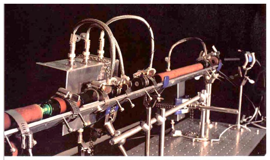
QUANTUM DEVICE generates and measures extremely faint flashes of polarized light, providing a secure way to transmit information [*see illustration on pages 56 and 57*]. On average, each flash consists of one tenth of a photon.
